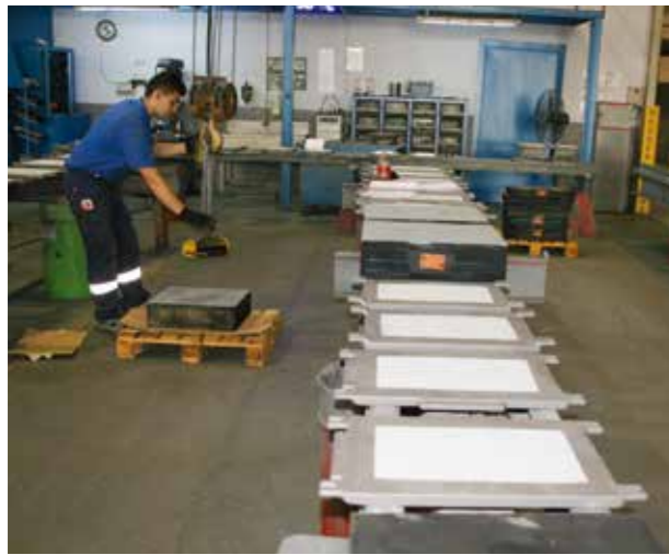
Elastomeric bearings during assembly
